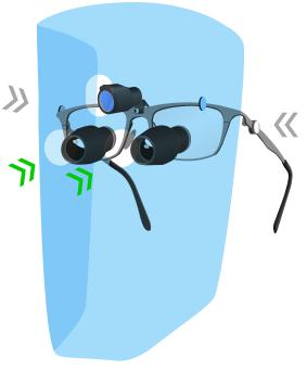
Align the two telescope holes and pass the telescopes through. **Bring** the left and right contact plates in proximity of the magnetic brackets to attach the visor into place.
